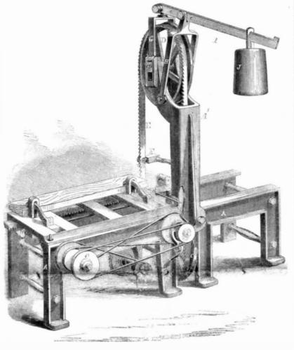
The principal reason why belt-saws are not in more general use is because, in many machines hitherto devised for carrying them, there has been something faulty about the arrangements which compensated for the expansion and contraction of the saw as it heated or cooled. That the belt-saw is really efficient and of great utility, a moment's consideration of the following points will show :
