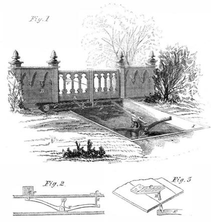
around two friction pulleys, G G, and it is attached to the gates by means of the two rods, d d, which rods move through a slot in the planks under the gates. When the carriage approaches the gates, the wheel passes upon the lever, C, at the right, which operates upon the rod, H, pressing down the lever, E, that moves the lever, D, and so moves the chain, F F, thus opening the gates; and as | above.
