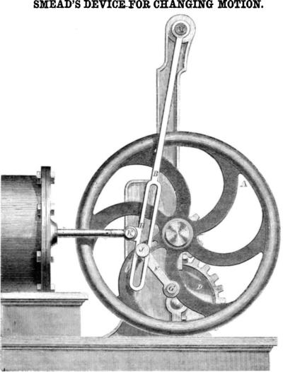
churns, where the turning of a handle attached to D gives an up and down motion to the dasher.
