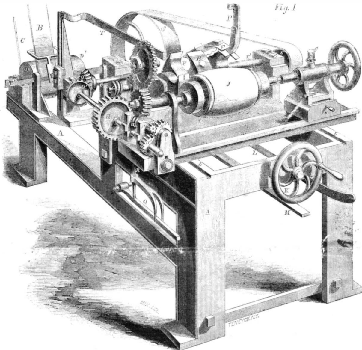
distance, and so produce a hub of any given diameter. When this point has been reached a rod that is secured to the plate, A', presses against the spring catch, P, and releasing it so that by the force of another spring the spiral, N'' is thrown or elevated out of gear with N' and the bedplate ceases to advance, at the same time the arm, Q, on a shaft that operated by a cam under A', is allowed to fall, and the rod, R, drops with it, bringing
