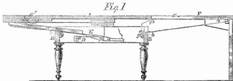
plates, F F', are brought to a level with the top, A, and the hooks, *g'*, fit over the projections, *h*, which are attached to the inner side
