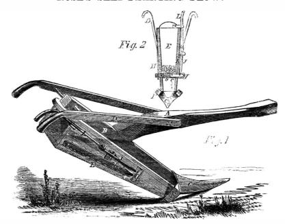
In the various departments of husbandry, tending a short distance below it, between sidered separate and distinct—two processes the invention which we are about to describe they have been joined, and sowing and plowing are performed at one operation. The invention is a seed-planting plow, and the inventor-J. H. Rose, of Versailles, Ill.-patented it August 17, 1858.
