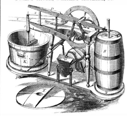
Either of these parts can be disconnected, | of the most convenient household appliances so that all or one can be used together, and the work of a household performed at once, or at separate times, as may be most convenient. The machine moves on castors, f, so that it can be easily transported from place to place, and on the whole it may be considered as one
