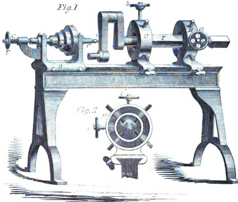
The tool, spindle and pulley are moved back and forth by the screw, G, and hand wheel, F. H H are two concentric chucks made to slide along the bed of the lathe, to which they can be secured in any position by screws, J; a and b are hand wheels to secure the object in the chuck after it has been adjusted by the screws seen in Fig. 2, which is a front view of a chuck.
