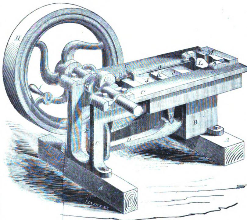
The great necessity which exists for a good and efficient stone-breaker is appreciated by all engineers, roadmasters, and lime burners, and at last the want has been supplied by Eli W. Blake, of New Hæn, Conn. The qualities necessary in a good and efficient machine are that it should be strong, durable, and compact, and that it should exercise a great force through a small space. The stone-
