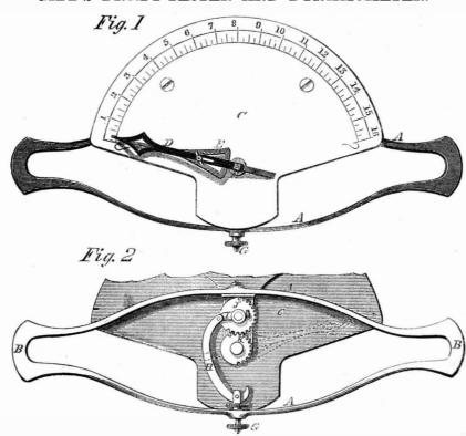
course, causes the pointer, D, to move round the dial, and the whole being proportioned and graduated correctly, the indicator, E, being only loosely placed on the axis, F, vibrates as the implement to be tested is drawn along, and indicates the average draft very
