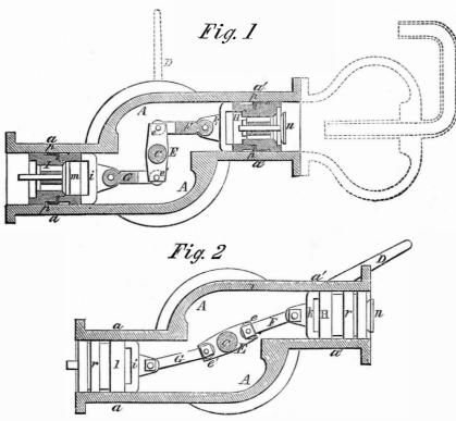
draws the water directly through itself from the entrance to the exit, and when placed perpendicularly draws the water in a straight column from the bottom to the discharge. It has but two valves, which can be taken out by simply taking the cap off the pump, and as a fire engine for farm houses or manufactories it is admirably adapted. It does not freeze, and is very cheap. The operation is easy and perfect, and it requires little power, as we can testify from a personal trial.
