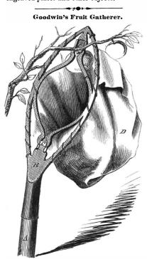
A great quantity of fruit is spoiled in the gathering, by being allowed to drop on the ground, or else the tree is much injured when they are violently pulled off by hand, as the small branches are liable to be broken. This simple little device, cheap and light, is one of the best we have seen for gathering fruit, neither spoiling it or damaging the tree. Any child can use it, and every one who gathers fruit should.
