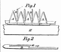
of a portion of the finger beam, H, guard fingers, B, and cutter, A, and Fig. 2 is a side elevation of one of the guard fingers detached, showing the opening, a, through the rear part of one side of the slot, to permit grass and leaves that may be carried into the slot by the cutters to work out. The claim in the patent reads as follows:—
