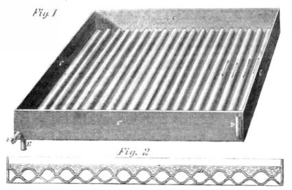
In the art of brewing it is essential that the wort, after being boiled with the necessary quantity of hops, and properly concentrated and rendered clear, should be cooled as rapidly as possible, to prevent acetification, or "fixing," as it is technically termed. The means employed at present to effect this object consists in having large shallow vessels constructed of wood, into which the liquor is poured,
