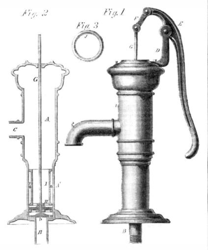
The great and common nuisance of pumps' packings wearing out, and the consequent stoppage of the pump, is by this invention almost entirely avoided, and that by a most simple and cheap contrivance. A ring of india rubber forms the piston packing, and as this as it wears is almost entirely self-repairing, it will last for a great length of time; and when it is actually worn out, another can be cheaply obtained and fitted in a few minutes.
