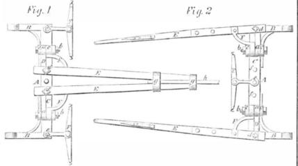
This invention is designed to render a carriage applicable for one or two horses with little trouble, so that a pair of shafts or a pole can be used on the one vehicle, at the discretion or convenience of the owner. How this is done will be seen by referring to our en-
