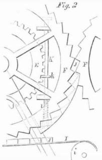
projection, k, and working up and down in suitable bearings; there is also a spring, l, which has a tendency to force the bar, K, up and keep it from the bricks.
