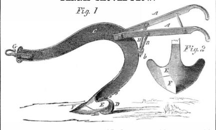
The adaptation of the plow to cultivating, as well as turning up the ground, is a valuable application; and those plows which break up the ground without leaving a furrow, are called from their shape, "shovel plows." They are used for cultivating cotton and sugar, and sometimes, when the ground is light, for breaking up, as in the sandy soil of South
