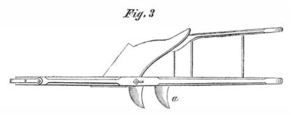
plow, through which the cutter is passed, and the bolts are put through the side of the plow, and passed through the flange inside. By taking off the bolts, the cutters are easily removed for sharpening, and they can again
