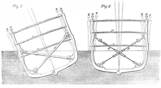
bilge, and between the upper and lower decks, C' and C. If, however, iron braces are preferred, they can be made and secured as seen in Fig. 2, where B, the brace or cross tie, is attached to the same places by plates strongly bolted, b, and these iron cross ties have screws and nuts, c, so that they can always be kept perfectly taut. E and F illustrate the vibra-
