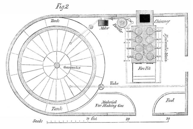
tributed in the usual way. As long as any volatile matters remain in the charger, an oscillating or dancing motion is kept up, by which it will be understood that a more thorough decomposition of the vapors is secured, since no wapor can possibly escape without passing between two red-hot surfaces;
