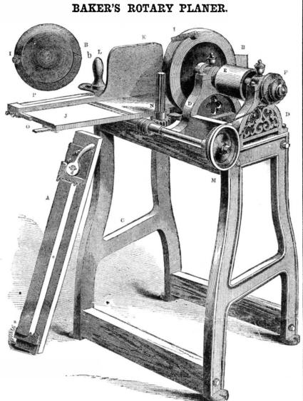
tions to any desired thickness, bevel or taper, at the rate of about thirty feet per minute, and also take the "wind" out, leaving the surface smooth, and the corners perfect. They are remarkably simple, and not liable to get out of repair.
