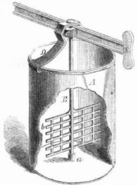
friction-band, C, there is a bar, E, by moving which backwards and forwards, a rotary motion is given to the spindle and grating, b. It will be seen that the vessel is provided with two lips which retreat enough to admit of D eing turned ease and facility.
