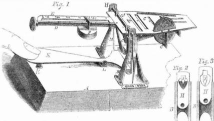
up when not in use, as it also allows J to rest on B. The balance, C, is supported from the beam, J, by the connections, G', and underneath, C, there is a rack, c, which is to support the coin in the measuring slit. It is applicable to all kinds of currency and can be graduated to suit any standard. The bearings of the knife edges may be applied to all kinds of balances for weighing diamonds or analytical purposes, and it is a cheap and useful little addition to every counting-house.
