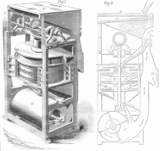
market, more or less smut, dust, chess, and other foul stuff; and in passing it through a smut mill, if the grain be the least damp, the smut dust, &c., is liable to adhere. It is absolutely necessary that the dust should pass out of the machine as soon as scoured from the berry, that the grain may not wallow in it.
