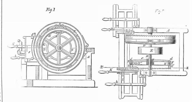
carriage, I, towards the saws by means of the lever, h. The two saws cut the fellies from the bolt exactly the shape they are required to be, and the thickness of the felly must depend on the number of rims between the saw, E', and the wheel, C, and fellies for wheels of different diameters may be cut by having a series of wheels, C, of various diameters. In Fig. 2, D | tained, and it facilitates their removal | when the patent was granted.
