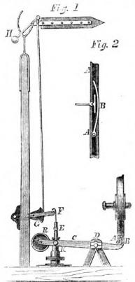
o each signal apparatus is applied pumping apparatus which communicates with the two ends of the two lengths of pipes or tubes, which respectively communicate forward and backward to two signal stations at distances from each station. The engine man and conductor of a train, on coming up towards a signal station will, by this arrangement, at once ascertain whether or not the preceding train has passed the next signal station.
