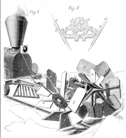
E have fans, f, on their ends placed obliquely to them, so as to throw away the snow up the bank during the motion of the machine. The flyers, G, on D, are at right angles with the arms, and have a point in the center, H, which bores the way through the snow while the flyers, G, throw it into f. The arrangement of C and D will be better understood by reference to Fig. 2, which is a section through | patented Nov. 10, 1857.
