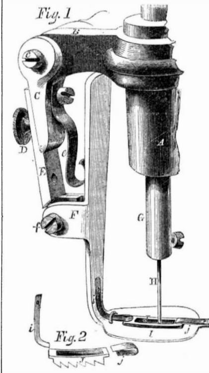
it a piece, B, to which is hinged the piece, C, by the screw, *c*. The screw, *D*, fastens E, and to it is hinged by the screw, *f*; the foot, *F*; this is kept on the cloth by the pressure of the spring, *e*. This foot has an independent mo-
