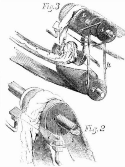
endless belt, G, being by it conveyed over the roller, L, seen in Fig. 3, when the scraper cuts it off, and lets it fall onto the endless band, H, which again conveys it into the mixer, C, from which it is taken by the endless belt, I,
