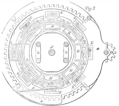
a circular inclined plane on which the bottom plungers, N, and under which, the top plungers, K, have to travel.
