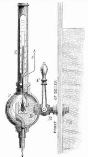
breaking. Part of the vessel, D, is broken away, to show the interior. E is the scale, and F a waste pipe, so placed that the excess steam or water can escape, and so allow the water in D to remain at its normal pressure; that is, at the same pressure as that in the boiler.
