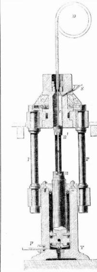
The manufacture of lead pipe by the ordinary method combines, like that of sheet lead, the double process of casting and elongation. Whatever may be the dimensions of
