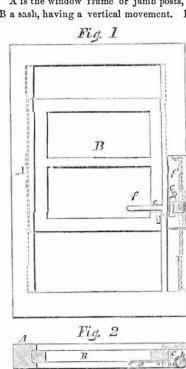
recess, f', in the frame, is placed the cord, E and to the side of B is attached the metal plate, C, whose outer edge is seen at a; another plate, D, is attached to it by an india rubber band, b, which passes through openings, c, in the plate. The outer edge of D is rounded, and the other has a shank, f, attached, which passes through a groove, e, in the stile of the sash.
