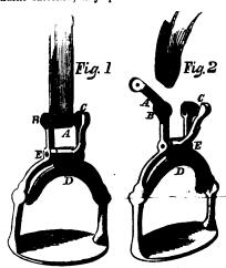
presses against this piece, D, will operate as a lever, and draw out the steel pin, C, and this liberates one end of the bar, A, which works freely at the joint, B, as seen at Fig. 2, and the stirrup will remain on the foot as both are freed from the saddle. This ingenious invention was patented Sept. 22, 1857.
