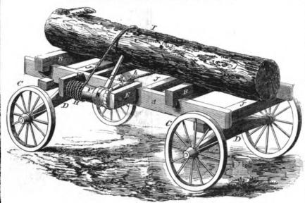
This carriage is intended for taking up logs from the forest or lumber-yard, and, by the apparatus connected with it, large pieces of timber are easily raised on to it. By reference to the engraving, the whole device will be appreciated.
