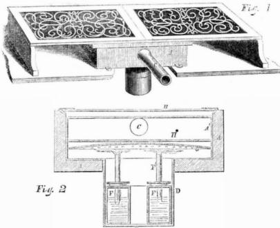
John W. Lefferts, of Brooklyn, N. Y., is the inventor of the simple means here represented for providing a source of heat, by which the feet may be warmed in sleighs or other vehicles. This stove, as it may be very properly termed, is inserted in the bottom of the vehicle, a principal portion being below the ordinary floor. Fig. 1 is a perspective view, and Fig. 2 a vertical section.
