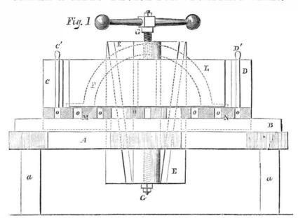
plate, E, and turning the screw, G; when the tire is clamped, the screw is turned in the opposite direction, and raising the block, E, forces together the blocks, CD, thus com-
