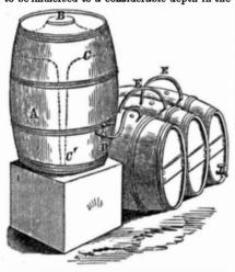
liquid. This arrangement prevents the possibility of the bag becoming entangled in any fold, and ensures its gradual and perfect expansion, as the liquor is withdrawn. D is a discharge tap or cock arranged in the ordinary manner.
