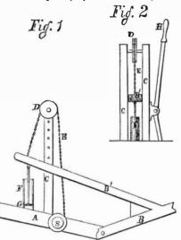
F, is attached to the under side of the arm B by a flexible joint or hinge and is provided with a valve on its lower side, said valve opening downwards. H is a clutch lever suspended by a suitable joint from standards C C.
