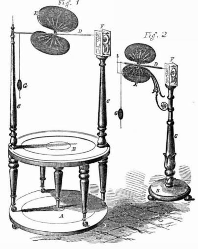
E E two broad thin wings of paper or other | platform, B, by the hand, the air is discharged suitable material, F strong clock-work, and in any direction at will. This device was patented June 9, 1857.
