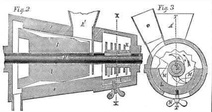
cave L may be inclined as much in the opposite direction, and the ears of corn allowed to drop much lower, so as to be exposed in a much greater degree to the action of K, and be torn in pieces much more rapidly in consequence.
