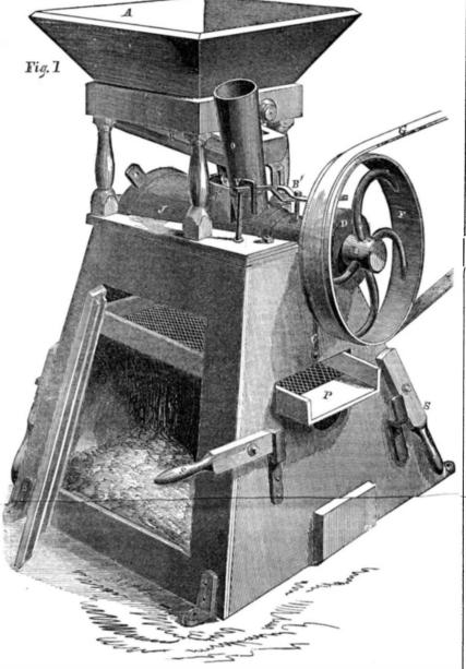
larger masses are fed when grinding whole ears. The ears dropped in O feed themselves down to the action of the teeth, K M, according to an adjustable device now to be described.
