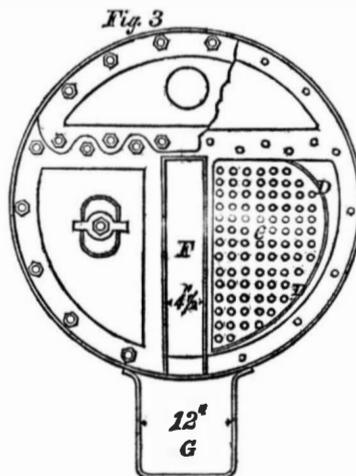
tirely expelled from the narrow spaces between the tubes, but the Dimpfel boiler allows no possibility of such an effect being produced, as a clear space always exists for the water to flow freely in at the front end, and to escape from the upturned ends at A, with great rapidity, whether in the form of water or steam. The current through these tubes has in some instances been so active as to carry a half-inch bolt through, and deliver it on the top of the crown sheet.
