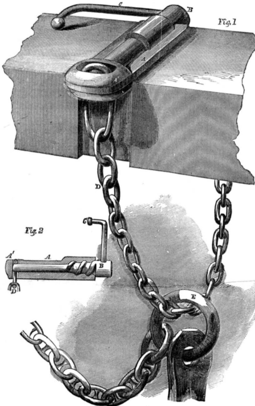
The accompanying engraving represents a simple device patented by Mr. John B. Holmes, of this city, on the 28th of April last, for the easy, rapid and safe release of an anchor when it is desired to let it fall. It is shown in perspective by Fig. 1, and in longitudinal section on a smaller scale by Fig. 2.
