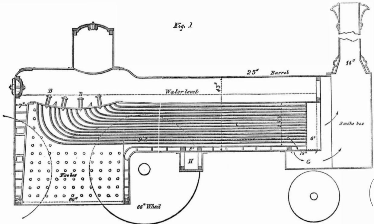
terior) and the far more heated products of combustion circulating within, so that both the nature of the metal and the higher temperature tend to make the tubes longer in proportion to the other parts than was the case when they were fitted to each other.
