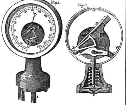
means indicates exactly the pressure. H is a | portion of the face of the dial is left open as slender spring, which acts on E with sufficient represented, in order to see that all the parts intensity to overcome the slight friction and insure its falling back, whenever the pressure mounted in a block, so that it may be traof the steam is lowered and B is depressed by the action of the stout coiled spring.
