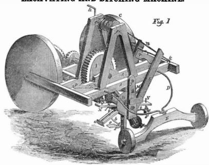
may be disconnected from springs, d, and at-The lever, P, may then be shifted, to throw action, and the scoops so arranged will cast their contents by the centrifugal action of the excavating wheel in a regular line, as the machine is drawn along. When the lifted earth is to be scattered at the side promiscuously, the scoops have different inclinations to discharge at different points of their circuit.
