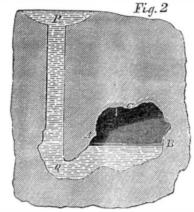
water must rise out of the pipe; an oscillation is produced; the water is pressed downwards from A to Q, and the steam, having room to escape, darts upwards, breaking through the column, and carrying along with it a great part of the water.
