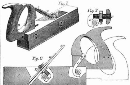
ventor of the ingenious means here represented for connecting and disconnecting the iron and the stock, and also for so attaching the handle, that it may be readily and firmly adjusted in two positions. The invention was plane irons by wedges as usually conducted, which are the tendency of the wedge to spring of the hand is applied to much better advan-
