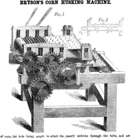
nub with the roots of the husks. The knife, I, is connected at its near extremity to the lever, H, and this lever is actuated by ranning in the oblique groove, g, in the surface of the pulley or cam, J, so as to receive a quick reciprocating motion.
