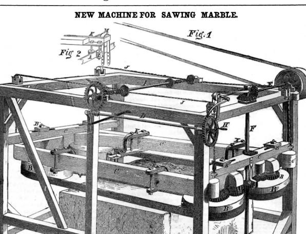
told that this machine cuts about three times | and there is no appreciable wear on their sur- | and operates with entire success. Further infaster than the common marble sawing appa- face. No difficulty is experienced in feeding ratuses. The endless saws may be driven at in the sand.
