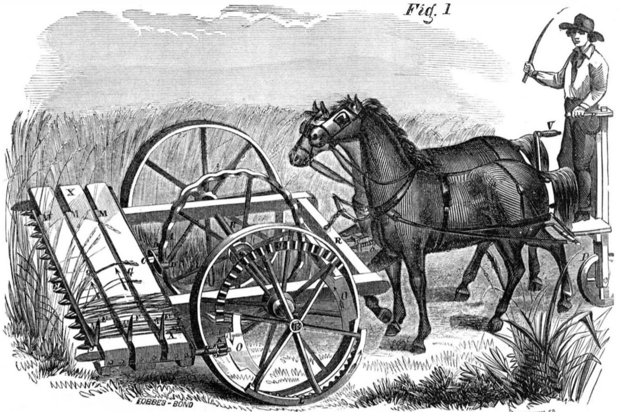
rection of the arrow, carrying along all the grain that has fallen in front of them, and throwing it off upon the ground; the teeth then disappear to rise at the opposite end of the platform and repeat the operation.
