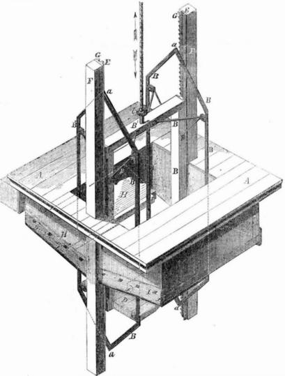
improved Safety Hatch, adapted to elevators, for the use of mills and warehouses, for nected by pawls with the rope, that in case which Letters Patent were granted to William | the rope should break, the pawls are instantly H. Thompson and Eustis P. Morgan, of Biddeford, Me., June 24th, 1856.
