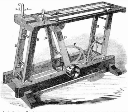
make it vibrate easily. J is a quadrant gauge any place, and can be set up in a few minutes. attached to the table for mitering. When not The parts are quite simple. It can be altered wanted, it may be quickly removed, by unscrewing its thumb button.
