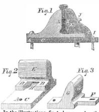
In the illustrations, fig. 1 shows an elevation of the chair when fixed; the dotted lines show the slide tongue and cotter. Fig. 2 shows a perspective view of the chair with slide withdrawn so as to admit of the rail being taken up or placed down; and fig. 3 shows a view of the slide and tongue part of the chair.
