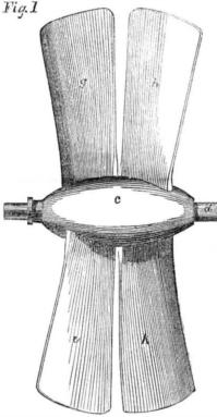
The patentee next describes how the blades are placed upon the boss, and also shows the position in which they stand with respect to each other when fixed, so as to produce the greatest amount of useful effect when in oper-
