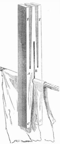
In securing clothes to the line, the lower jaws are extended to their fullest extent, by pressing the prongs, F, together, and the jaws,
