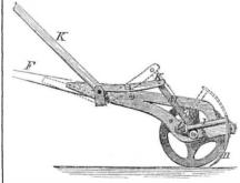
H are the raker teeth, made in curved form and attached to arms, I, which are pivoted at L. M is a connection rod which unites arms, I, with lever, K. By pressing down lever, K, the rake arms, I, with the rake will be elevated, and vice versa. A pin may be used at any convenient point to fasten K down, and keep the rake elevated, when desired.
