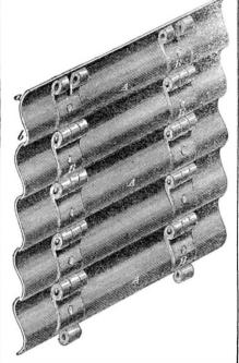
A represents the slats of the shutter connected by hinges, B, which are secured to the backs of the slats.
