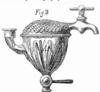
of dirt on one side of the filtering material. The present improvement overcomes that difficulty, in a great degree. Fig. 3 shows the external appearance, which may be rendered highly ornamental. The invention is applicable to large cistern reservoirs, and the purification of rain water. The form here shown is chiefly intended for city use. Patented July 1, 1856. Apply to the inventor, 835 Broadway, N. Y., for further information.
