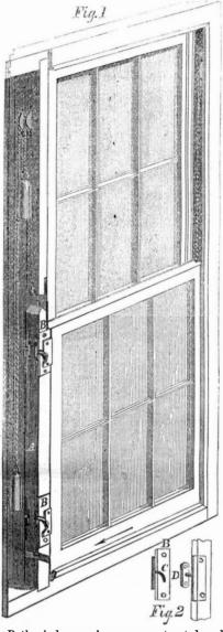
Both window sashes are constructed and hung with weights in the usual manner. One portion of the stile, A, is made movable; its ends are furnished with metallic plates, B B', in which curved slots, C, are cut. Button headed pins, D, attached to the frame, fit the slots, C. See fig. 2.
