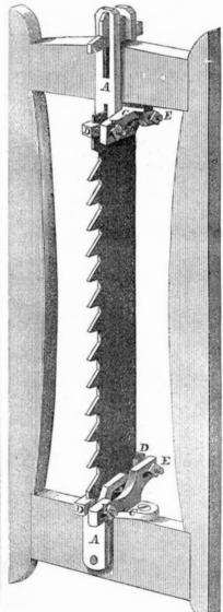
Each end of the saw is held by two stops one in front and one behind. By turning the nuts, E, which secure the stops to the saw, the stops will be changed in their position and the saw adjusted accordingly. The common method of holding saws is to drive wooden wedges between the saw and the stirrup.
