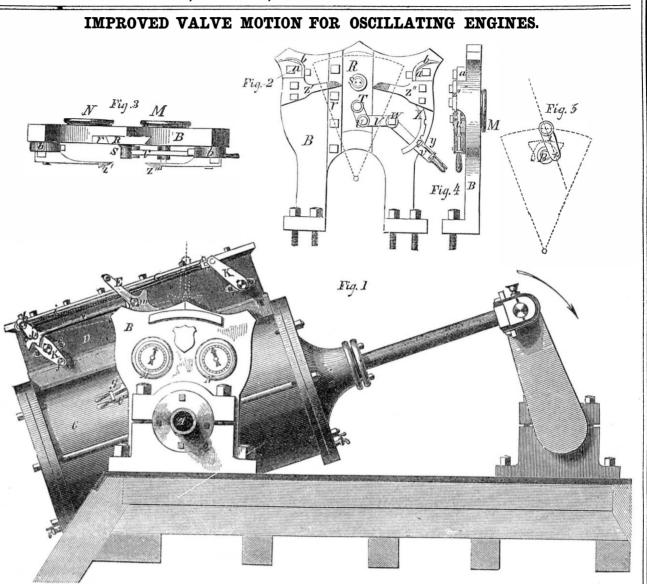
stand, B, to operate upon two arms, 2 2, at-1 thest points of oscillation in either direction, | oscillating engines for a long time, and they tached to the rocking piece, E, for the pur- one or other of the arms, 2, which are beveled pose of operating the rocking piece to move on their outer side, presses back the catch, Z' the values to shut off steam from the ports.
