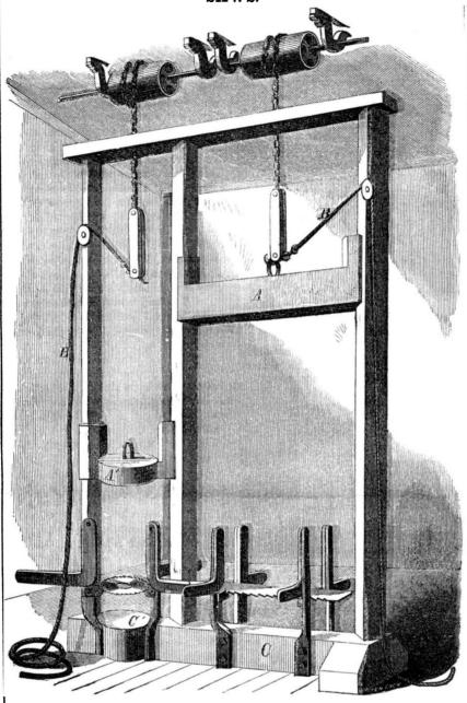
Improvement in the Manufacture of Saws. The usual method of tempering saws is to heat and then dip them in oil. This process is slow, laborious, and costly; it is also disadvantageous, because the saws become warped, and require to be hammered up straight again by hand.
