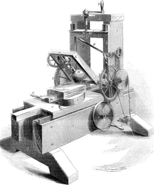
there are, in reality, several. They are of spherical shell-shape, placed one within the other, but all attached to the shaft, J.
