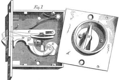
The acompanying engravings are illustra- | shown in fig. 1, the latch, D, is fastened down, tive of the improved Latching Lock patented in this country by Mr. Edmund Field, of Green-key H in direction of the arrow, and bolt C wich, Ct., July 3rd, 1855, and in Europe April, 1855.
