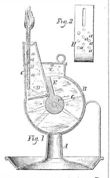
of being forced close to it by the piston. Th holes or apertures, a, afford a free communication of the lard to the wick, causing the lamp to burn a considerable time without operating the piston, as the lard will be in contact with the wick as far up as the holes or apertures, a, extend. The valve, D, sustains the lard in the wick tube when the piston is moved back to refill the chamber, B. Owing to the method o keeping the lard close to the wick in this lamp, it gives out a brilliant flame.
