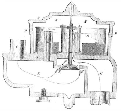
The accompanying engraving is a vertical section of an apparatus for regulating the supply of gas to burners, for which a patent was granted to Walter Kidder, on the 12th of October, 1852.
