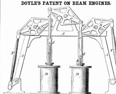
The accompanying figure represents a new arrangement of two beam engines connected to drive parallel shafts, for which a patent was granted to Thomas Doyle, of this city, (N.Y.) on the 6th of last November.
