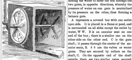
This figure is a perspective view, showing the inside, of an improved balance water gate, for which a patent was obtained by E. N. B. Section openings or slits,  $b^2$ ,  $b^2$ , are cut in Moore and J. H. Hanyan, of Lenoxville, Pa., | the sides of the box, and the gates cover them. on the 24th of July last. The nature of the invention consists in When the gates close them, no water enters
