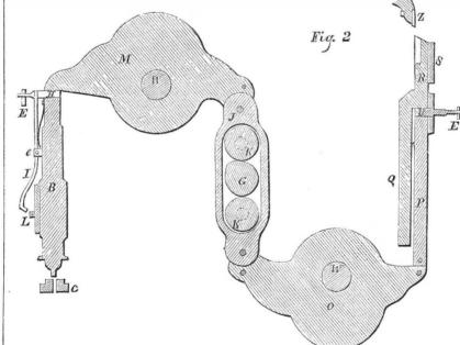
are springs to throw back the hand levers.- ing in contact with the top of casing, a. Th b c d are necessary gearing and fly wheels for slide, H, is moved between B and M, and ope giving motion to the machine.
