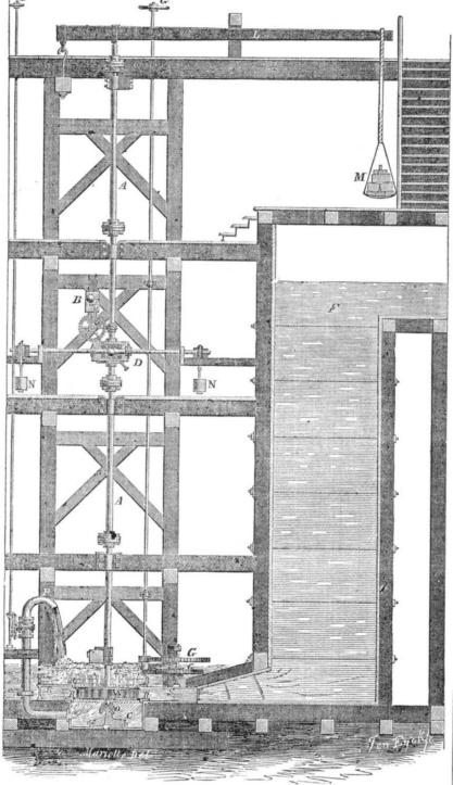
Reuben Rich's patent Center Vent Wheel with | plain, and will be readily understood. a cast iron scroll, to which is applied Winters' Hydrostatic Chamber. This view represents taining the power of the wheel, is also repre-
