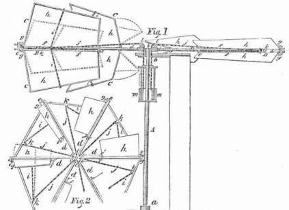
The accompanying engravings represent an improvement in Windmills for which a patent end of it runs in a suitable step, a, and its upwas granted to J. S. Morgan, of Highland, per end is fitted in a suitable bearing, b, at-Madison Co., Ill., on the 17th of July last. Fig. tached to proper frame-work. To the top of 1 is a side elevation of the windmill, and fig. 2 the shaft there is attached a hub or boss, c, to is a top view of it. Similar letters refer to like parts.
