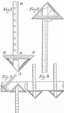
The application of the instrument as a graduated rule, T-square, and try-square, will be easily understood by inspecting fig. 4.
