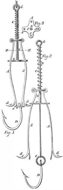
bring the barbs or hooks d d, between his jaws, and then pulls slightly upon the bait hook, D, it will be sprung, as shown in fig. 2, or unset, and the barbs, by the action of the spiral spring, C, caused to move laterally from each other, and consequently take into the top, bottom, and sides of the fish's mouth, and confine him securely, and thus relieve the bait hook of nearly all the strain.
