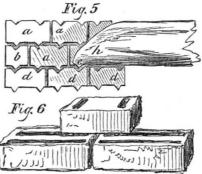
"It will be perceived at once that in bricks made upon this plan, the improvements will consist. 1st, in the greater security and strength of the walls locked and bound together by this device. 2nd, the bricklayer is enabled to lay several courses without the use of the line, and with much greater rapidity and accuracy than with common brick, it being scarcely possible to go wrong; and, 3rd, the spaces for mortar between the bricks are necessarily uniform, exact, and equal.
