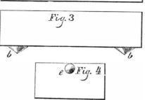
The annexed figures are views of an improved brick, for which a patent was granted Ohio, at Columbus, Sept. 18-21. to Levi Till, of Sandusky, Ohio, on the 19th of Pennsylvania, Sept. 25-28. grooves upon the top, and with projecting conical spurs upon the bottom and upon one of its ends.
