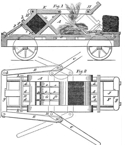
Hay Press, for which a patent was granted to Pells Manny, of Waddam's Grove, Ill., on the lower ends of the doors, H, and the doors, I, 17th of April last.
