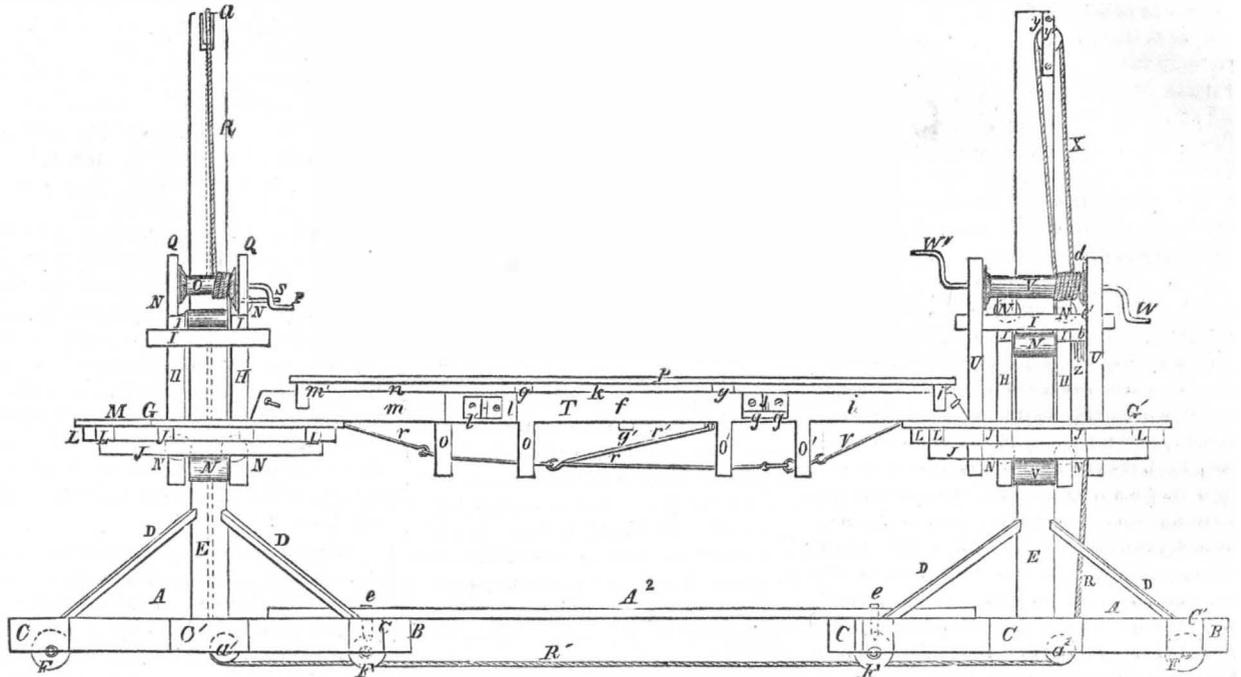
workmen to walk on. In using this staging the workmen on the platform, G, can raise or lower it by turning the crank, P, and the workmen on the platform, G', can raise or lower both platforms at the same time by
