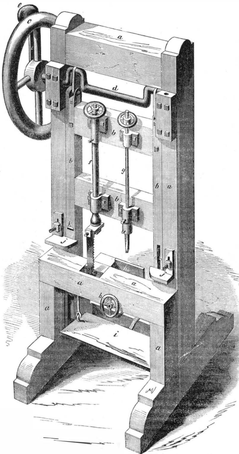
The annexed engraving is a perspective view of an improvement in the above named machines, for which a patent was granted to Elihu Street, of Montville, Ct., on the 20th of March last. The nature of the invention consists in the combination of certain tools used by carpenters in the manufacture of doors, sash, and blinds in such a manner as to avoid loss of time occasioned by removing the work from one machine to another.
