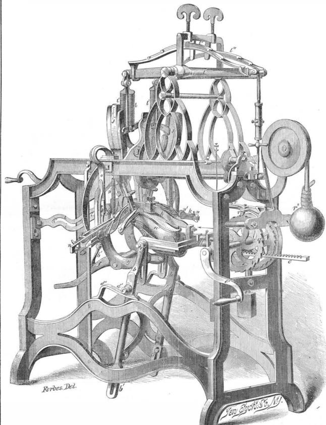
standards are fed forward, the shoe frame is raised on them by the said fixed curved i i, guides the front end of the shoe frame, by a pin on each side of the frame, running in each slot. This curvature of the rail and slot is made to raise the shoe to the exact and proper distance under the awl and peg-driver, and gives the shoe the proper angle to receive and drive in each peg. All these devices are therefore very correct and skillfully arranged.
