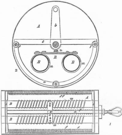
provement for preventing incrustations in steam boilers, and increasing the production of steam, for which a patent was granted to John McMul- continually mixed with the water, and are len, of the city of Baltimore, Md., on the 20th of last May (1854.)
