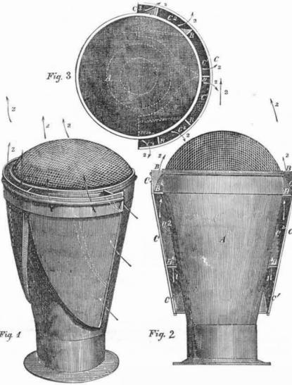
back of a new Spark Arrester; fig. 2 is a front train, the air is made to flow upwards, and as elevation, and fig. 3 is a top view. The same letters indicate like parts.
