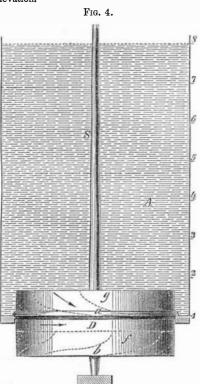
In fig. 4, A is a cistern 8 feet in depth, f, is a turbine wheel,  $\,g\,$  the stationary guides placed over it; a is the lower part of one of the guides, b an issue of the wheel, and S, the shaft. The dotted lines show the form and position of the guides and buckets. The dart in the space D, between the guides and wheel, indicates the direction of the water.
