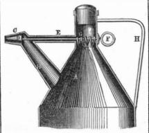
The annexed engraving is a perspective view of the ordinary decanting vessel, with a sectional view of the tube, showing Nichol's improvements attached.
