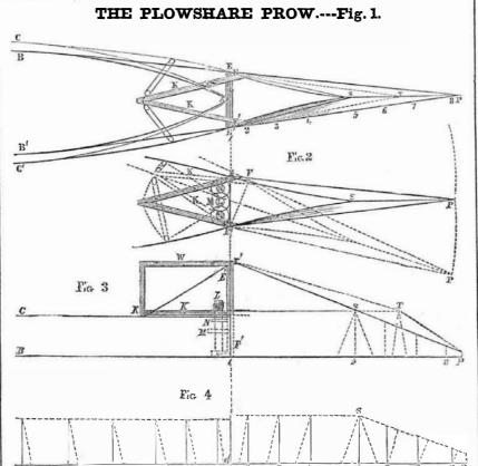
EXPLANATION OF THE ENGRAVINGS.—To a | tom; the long line, P A B, fig. 3, is the same tom, it is proposed to add a Wave-line Sow of one-fourth the length of the boat, with a base of one half of the boat's medium beam say 183-4 feet.
