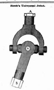
This Joint was invented by Dr. Hook, and exhibits a decided improvement over the old Universal Joint for coupling shafts that are inclined to each other This will form a useful accompaniment to the above engraving as exhibiting on an enlarged scale, the manner in which the piston rod and the connecting rod b, are united together. A and B are two shafts
